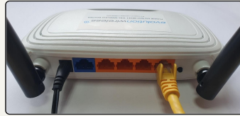
The other end of the yellow cable goes into any of the orange ports.
